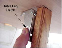
5. Remove the table from the wall support bracket by lifting the end of the table.
