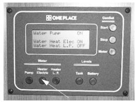
Electric Water Heater Switch (Located on OnePlace<sup>®</sup> monitor panel)
