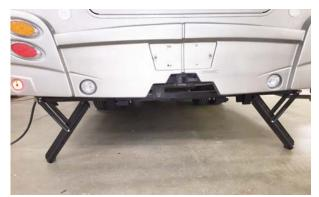
Stabilizing Jacks Shown in Down Position -Typical View
