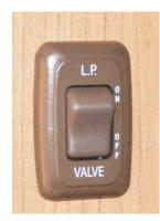
Main Tank Valve Switch (Located near monitor panel area) -Typical View *NOTE: The propane tank is equipped with an automatic 80% stop-fill device.*
