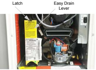
Easy Drain Lever (Located behind water heater access panel on exterior of coach)
