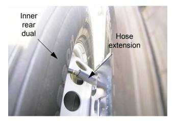
4. Using the hose extension as a remote handle, unscrew the valve stem cap (retaining cap in the end of the hose extension).
