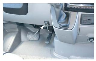
Radio Power Switch (Located on lower dash area)
