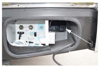
Single Solar Port (Located inside rear driver side exterior compartment)
