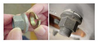
Steel Wheel Lug Nut and Washer (Hex Flange Nut with Split Cone Washer)
