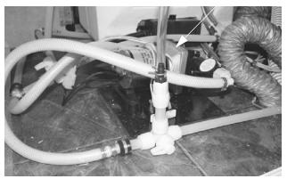
Water Pump (Located in backwall compartment. Remove side panel to access) -Model 24V shown
