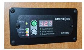
Inverter Control Panel (Located near monitor panel) -Typical View
