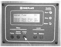
Propane Gas Water Heater Switch (Located on OnePlace<sup>®</sup> monitor panel)
