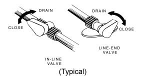
Water Tank Drain Valve
