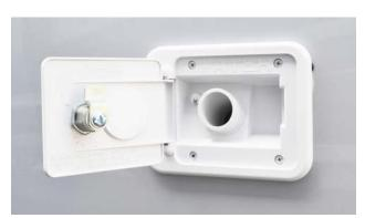
Water Tank Gravity Fill -Typical View
