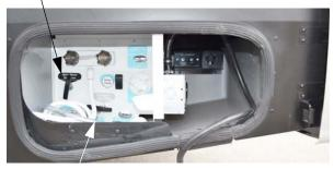
• **2nd** - Pull Gray Waste Tank Drain valve to drain Gray Water (sink/ shower) tank – then close.
