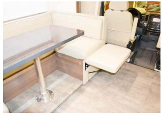
2. **To Store:** Pull footrest all the way up until the locking arms release and lower into stored position.
