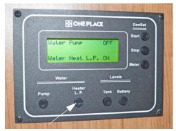
Propane Gas Water Heater Switch (Located on OnePlace<sup>®</sup> monitor panel)
