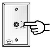
Digital Antenna Power Switch (Located in an overhead cabinet or mounted on a wall near the TV)
