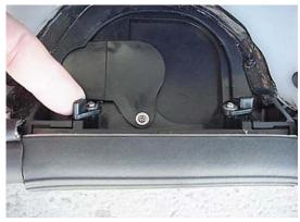
· Swivel the latch aside and drop the hatch
