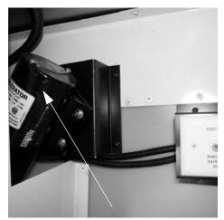
Waste Pump (Located behind water service center accessible through utility compartment) -Typical View
