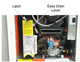
Easy Drain Lever (Located behind water heater access panel on exterior of coach)
