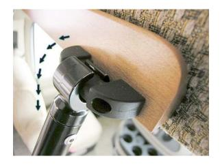
NOTE: Ensure top of ladder is properly engaged onto retainer brackets and ladder is resting firmly on floor before using.
