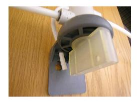
4b. **If Equipped with Culligan Cold Water Filter:** Remove the filter canister from the Cold Water Filtration System under the galley sink and discard the filter cartridge. After emptying the canister, remount it onto the filter assembly and continue the Blow-Out Procedure.
