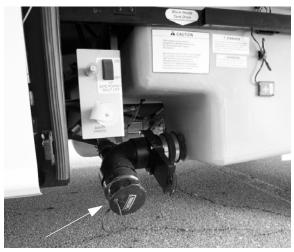
Sewage Drain Outlet/Dust Cap (Located in driver side compartment) -Typical View
