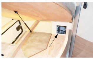
Water Pump (Located behind removable access panel below bed) -Model 24J shown
