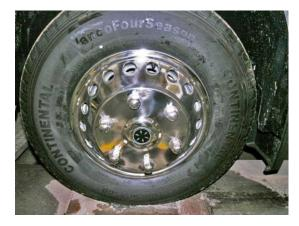
The wheel on your coach has a push on liner which is removed similar to a hubcap. Remove the covers by carefully prying the perimeter flange away from the wheel flange.
