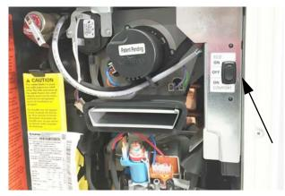
Water Heater Mode Switch (Located behind water heater access panel on exterior of coach)
