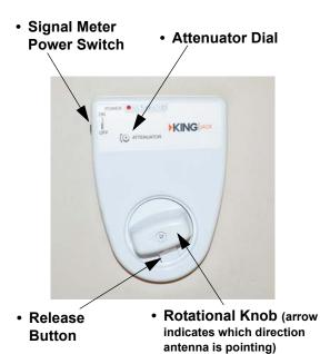
Digital Antenna Signal Meter (Located on ceiling)
