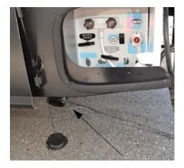
Sewage Drain Outlet (Located on the underside of water service center) -Typical View
