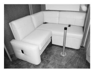
8. Place dinette table onto the pedestal leg, ensuring the receiver on the bottom of the table is fully seated on the pedestal leg.
